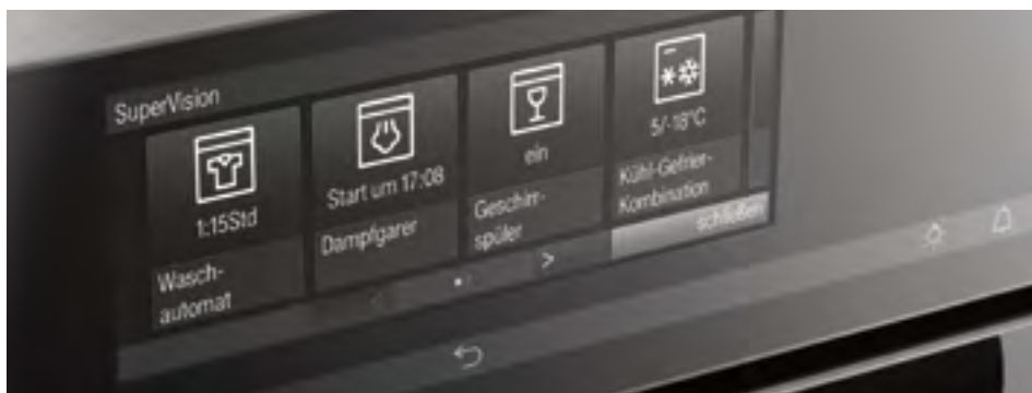
For the SuperVision application, the oven display provides information about the Miele appliances connected up to the system.
