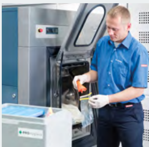
After the wash cycle: The orange-coloured bioindicator is removed from the drum and sent for testing in a sterile, polythene bag.
