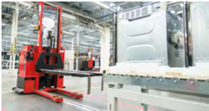
Finished ovens are automatically transferred to the packing station.
